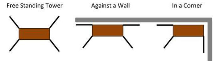
When moving a tower plan the route and be aware of hazards both on the ground and up above, adjust the top clamp of the stabilizers and lift the rubber foot no more than 25mm from the ground, release the braked wheels and push the tower to required position. Once in position reapply brakes, level tower and reposition all stabilizer feet to ensure firm contact with the ground.
